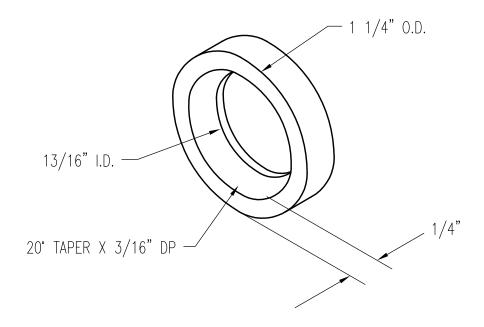
THIS WASHER IS USE ON 3/4" ROD ENDS ON CAST BELT ASSEMBLIES
