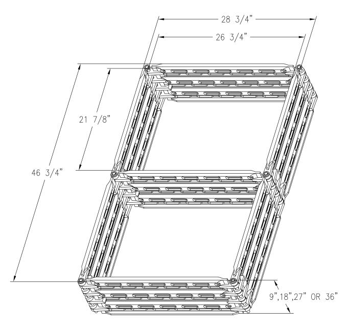
BASKET ASSEMBLY DESIGNED TO FIT CASTALLOY CC-2001 SERIES 30" X 48" RAIL TRAY ASSEMBLIES. ALSO, CAN BE MODIFIED TO FIT OTHER 30" X 48" TRAY ASSEMBLIES. HEAVY WALL AND LIGHT WALL AVAILABLE.
